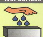
Wet the surface of blocks before applying mortar.
